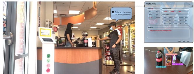
Figure 1: When the user wears HoloLens 2 and stands by the side of the cashier, the user clicks the camera button to capture current objects on the desk. In this scenario, there are three objects on the desk: soda, coffee, and water. After the captured image is processed on the server, the detected objects, the generated keywords, and the generated sentences will be shown in front of the user via an AAC interface visualized by HoloLens 2. As the user clicks the prices keyword, the sentence “what are the prices of these groceries?” is shown. The user clicks this sentence to trigger our application to speak it accordingly.
