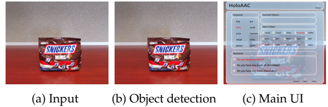
Figure 11: Object detection failure. (a) The image captured. (b) The object detection result. It did not succeed as nothing was segmented in the previous step. (c) The main UI showing that the chocolate and have keywords were selected by the user. The target sentence Do you have chocolate? was selected and spoken.
